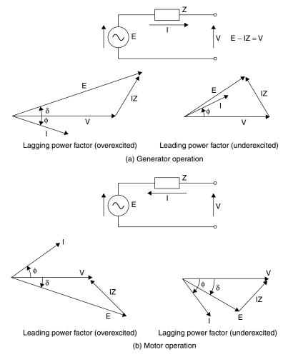
Fig. 1.27 Steady-state equivalent circuit and vector diagram.
