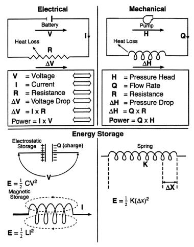
Fig. 1.6 Electrical-mechanical equivalence.
