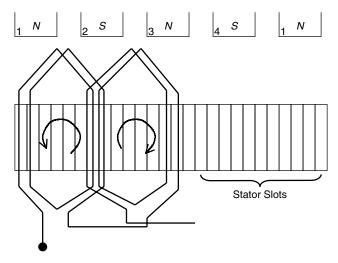
**Fig. 1.21** "Developed" view of a four-pole stator, showing the slots, the poles, and a section of the winding. The section shown is of one of the three phases. It can be readily seen that the winding runs clockwise under a north pole, and counterclockwise under a south pole. This pattern repeats itself until the winding covers the four poles. A similar pattern is followed by the other two phases, but located at 120 electrical degrees apart.
