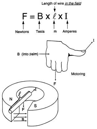
**Fig. 1.14** The Ampere-Biot-Savart law of electromagnetic induced forces as it applies to electric rotating machines. Basic numerical relationships and a simple rule are used to determine the direction of the induced force.
