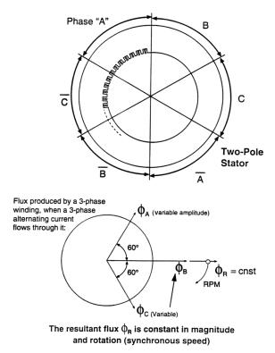
**Fig. 1.23** Production of stator rotating field. A constant magnitude and constant rotational speed magnetic flux is created when three-phase balanced currents flow through a three-phase symmetrical winding. In a two-pole winding, however, any the same result applies for any number of pairs of poles.
