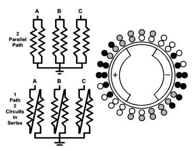
**Fig. 1.22** Schematic view of a two-pole generator with two possible winding configurations: (1) A two parallel circuits winding, (2) A two series connected circuits per phase. On the right, the three phases are indicated by different tones. Note that, some slots only have coils belonging to the same phase, while in others, coils belonging to two phases share the slot.
