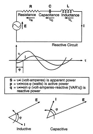
**Fig. 1.9** Alternating circuits (resistive—Inductive—Capacitive). Here the sinusoidal voltage **E** is applied to a circuit comprised of resistive, capacitive, and inductive elements. The resulting angle between the current and the voltage depends on the value of the resistance, capacitance, and inductance of the load.
