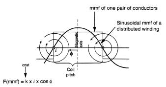
**Fig. 1.20** Schematic cross section of a synchronous machine with a cylindrical round-rotor (turbogenerator). This is the typical design for all large turbogenerators. Here both the stator and rotor windings are installed in slots, distributed around the periphery of the machine. The lower part shows the resulting waveforms of a pair of conductors, and that of a distributed winding. The formula giving the magneto-motive force (mmf) created by the windings.
