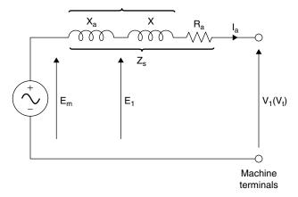
**Fig. 1.26** Steady-state equivalent circuit of a synchronous machine. X = leakage reactance,  $X_a =$  armature reaction reactance,  $X_s = X_a + X =$  synchronous reactance,  $R_a =$  armature resistance,  $Z_s =$  synchronous impedance,  $V_1(V_t) =$  terminal voltages, and  $E_m =$  magnetizing voltage.
