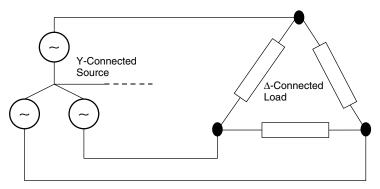
Fig. 1.12 A "Wye-connected" source feeding a "delta-connected" load.
