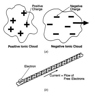
**Fig. 1.5** Electricity. (a) Ionic clouds of positive and negative currents. The positive clouds are normally atoms that lost one or more electrons; the negative clouds are normally free electrons. (b) The flow of electrons inside a conductor material, for example, copper.
