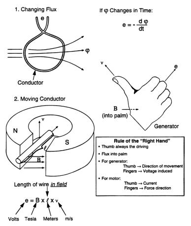
**Fig. 1.13** Both forms of Faraday's basic law of electromagnetic induction. A simple rule (the "right-hand" rule) is used to determine the direction of the induced voltage in a conductor moving across a magnetic field at a given velocity.
