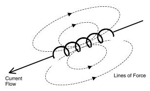
**Fig. 1.4** Schematic representation of a magnetic field produced by the flow of electric current in a coil-shaped conductor.
