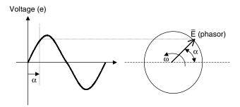
**Fig. 1.7** A phasor **E**, that can represent the voltage impressed on a circuit. The phasor is made of a vector with magnitude proportional to the magnitude of **E**, rotating at a constant rotational speed  $\omega$ . The convention is that phasors rotate counterclockwise. The vertical projection of the phasor results in a sinusoidal representing the instantaneous voltage e existing at any time. In the graph,  $\alpha = \omega \times t$ , where t is the time elapsed from its zero crossing.
