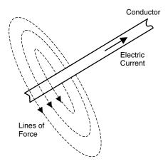
**Fig. 1.3** Schematic representation of a magnetic field created by the flow of current in a conductor. The direction of the *lines of force* is given by the "law of the screwdriver": mentally follow the movement of a screw as it is screwed in the same direction as that of the current; the lines of force will then follow the circular direction of the head of the screw. The magnetic lines of force are perpendicular to the direction of current.
