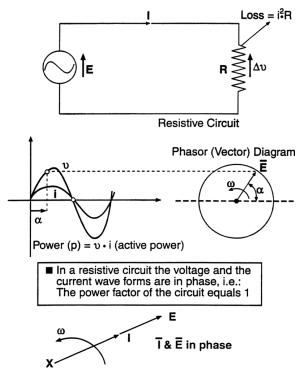
**Fig. 1.8** Alternating circuits (resistive). Schematic representation of a sinusoidal voltage of magnitude E applied on a circuit with a resistive load R. The schematics shows the resultant current i in phase with the voltage v. It also shows the phasor representation of the voltage and current.
